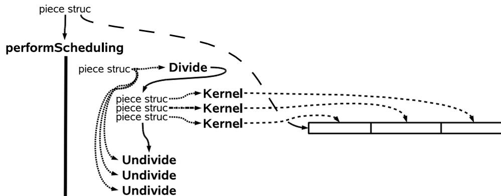
**Figure 2.** A representation of the call structure plus data structure for the DKU pattern implemented in an OO paradigm. Solid lines represent data flow, coarse dashed lines represent pointers, medium dashed lines represent side effects, and fine dashed lines represent method calls invoked on an object. The thick line below “performScheduling” demarcates the activity that takes place during the method call.
