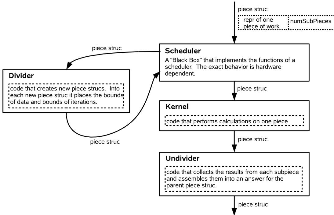
**Figure 1.** The flow of data through the elements of the DKU pattern
